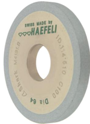
Our aggressive SHARKLINE with a lot of bite for CNC creep feed grinding. Large depths of cuts, high feeds, small grinding pressure. Wet grinding with oil is recommended. For grinding of flutes, flanks, external surfaces und similar grinding tasks where a lot of material has to be removed. Optionally available with a body reinforced on one side (type 3A1). Can be wire dressed (EDM).
