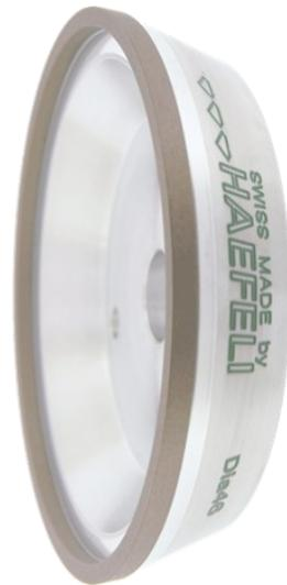
Stable tapered cup wheel which can be used at the same time as a profile wheel since open geometries such as rake faces can be ground with its point angle. Compared to 14E1D wheels (→ 2-12), they have a broader point angle and a more massive body which is an advantage when grinding materials that create high grinding pressures and when a lot of material has to be removed.
