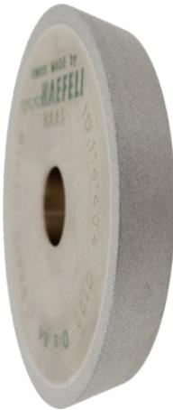
Our aggressive SHARKLINE with a lot of bite for CNC creep feed grinding. Large depths of cuts, high feeds, small grinding pressure. Wet grinding with oil is recommended. For grinding of flutes, rake faces, flanks, outer diameters, point thinning and the like on CNC machines. Very high stock removal rates. Can be wire-dressed (EDM).
